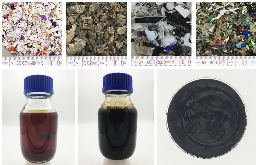
Figure 15: Below: Product spectrum from an industrial oiling plant. Left: Light fraction, middle: Heavy fraction, right: Wax. Top: Typical feed material from this plant [51] (photos: FH Merseburg).
