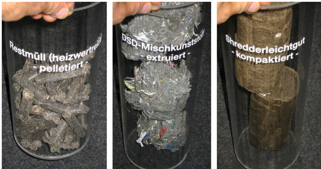
Figure 11: Input materials at SVZ Schwarze Pumpe, Germany (2003). Left: Pellets made from processed residual waste, middle: extrudate from DSD plastic waste, right: briquettes from SLF.
