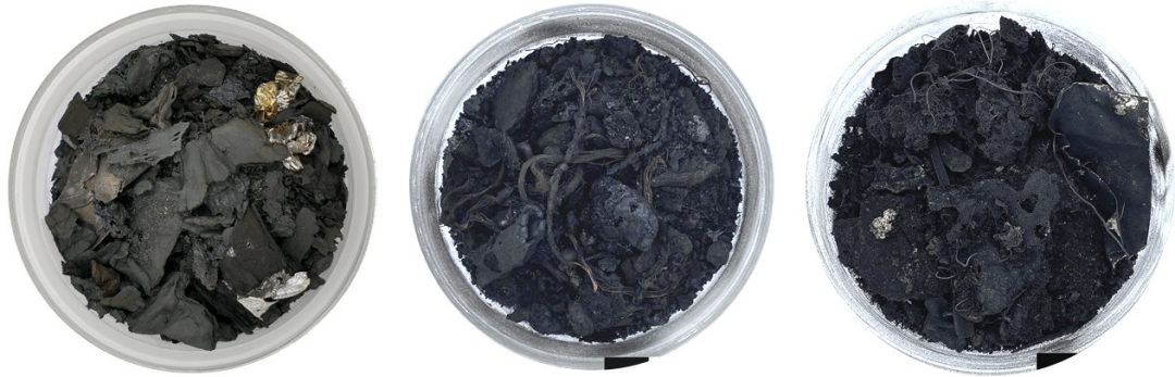
Figure 17: Solid residues from pyrolytic treatment of plastic waste fractions. Left: Mixed plastic waste from packaging, middle: Shredder fraction from WEEE, right: SLF from EOL vehicles [51] (photos: F. Roemer).
