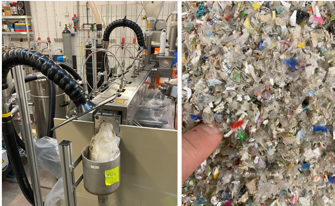
Figure 3: revolPET pilot laboratory plant and typical input material.
