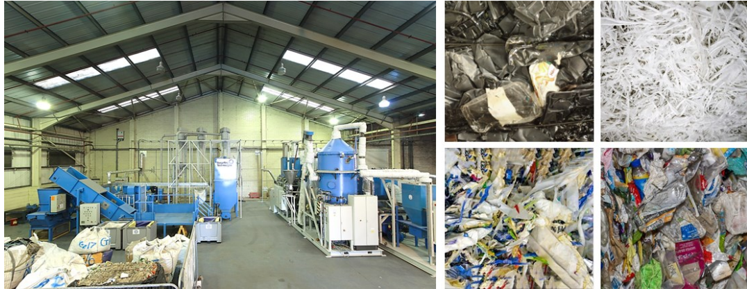
Figure 8: Pyrolysis pilot plant of Recycling Technologies in Swindon, UK and typical input materials.
