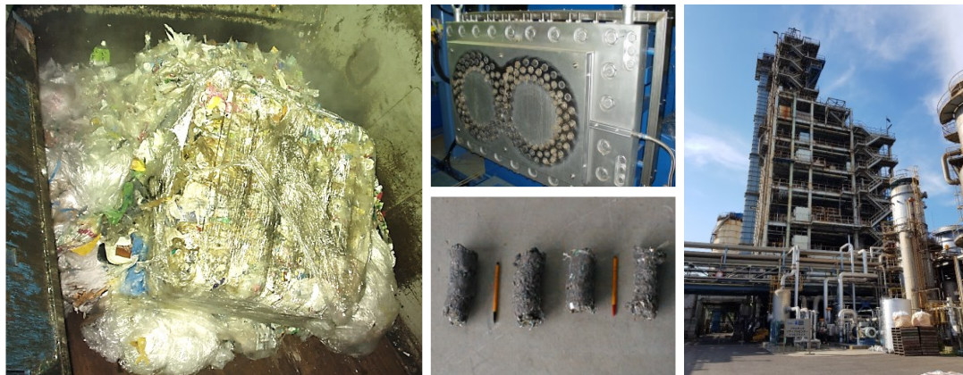
Figure 9: Gasification of plastic waste at Showa Denko, Kawasaki Japan (2017). Left: input material, middle: extruder for preparation of plastic waste and produced extrudates, right: gasification reactor according to Ebara UBE process.
