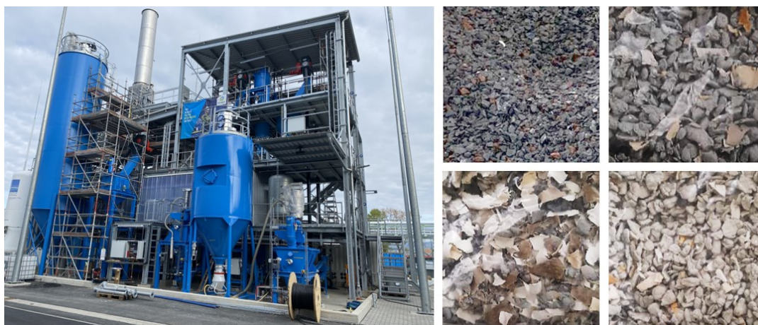
Figure 7: Pyrolysis pilot plant of Arcus Greencycling Technologies in Frankfurt Hoechst, Germany and typical input materials [62].
